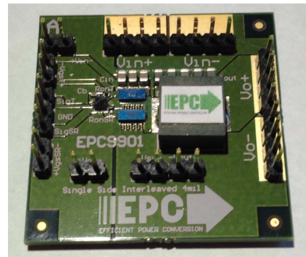
Experimental Prototype L_{LOOP} \approx 0.4 \text{ nH}
